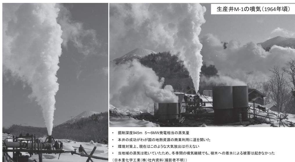
Fig.8 Steam discharge from well M-1.
